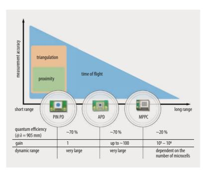
Each different type of photosensor supports a specific lidar system
