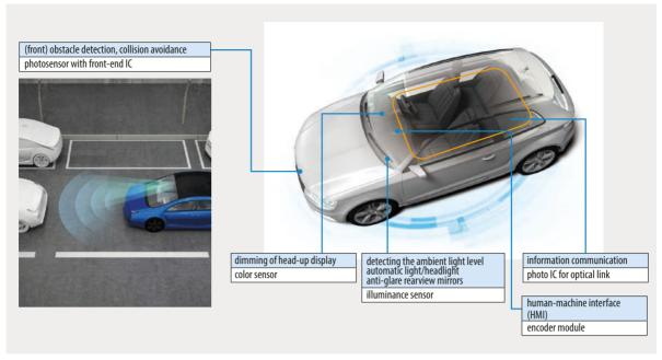
The photosensor with front-end IC optically measures the distance to the front car return and controls the distance to the vehicle.
